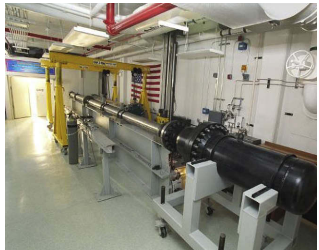
Fig. 3. The NASA Glenn Research Center Ballistic Impact Laboratory gas gun.
