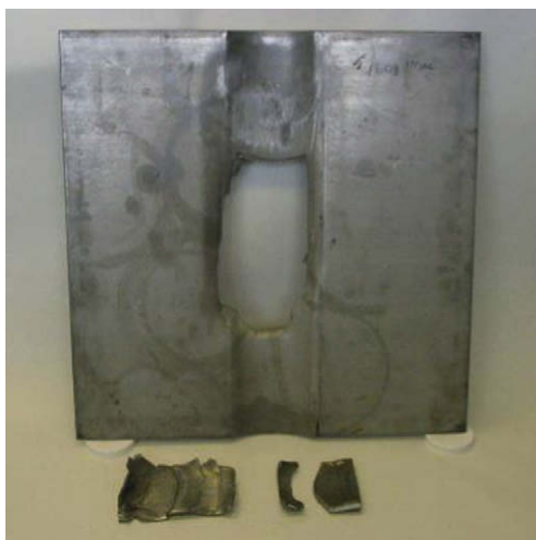
Fig. 15. Curved at 490 m/s (1608 fps).
