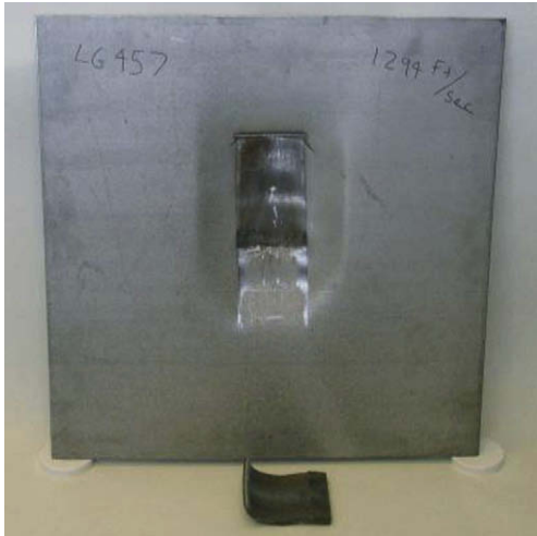
Fig. 10. Flat at 394 m/s (1294 fps).
