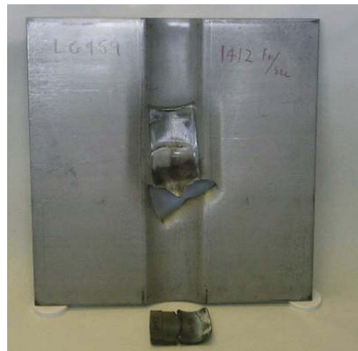
Fig. 13. Curved at 430 m/s (1412 fps).
