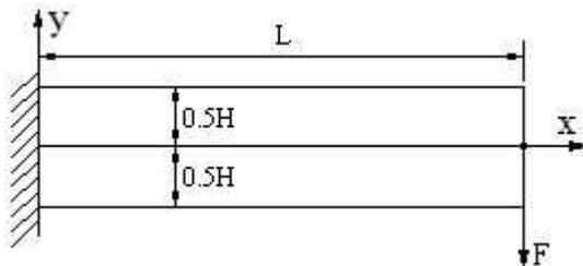
Fig. 2 Bending of a cantilever
