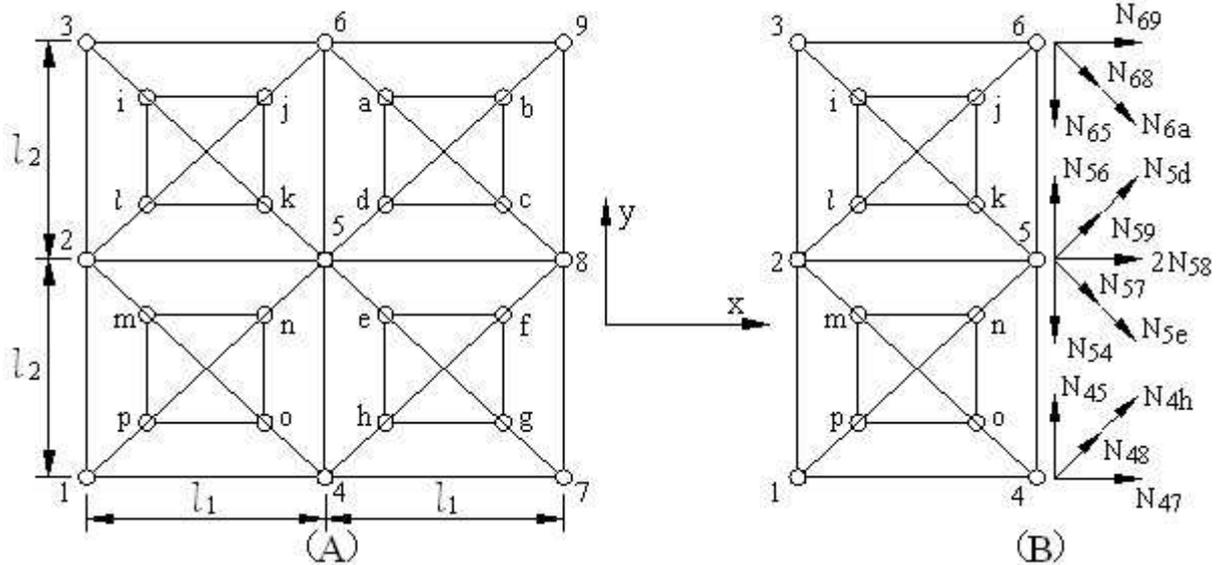
Fig. 1 Analysis of strain and stress at a point: (A) four new elements around node 5; (B) stresses from axial forces of bars
