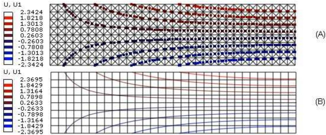
Fig. 4 Displacement contours in the x-direction of the cantilever: (A) the new element method; (B) the finite element method
