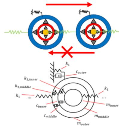
Lattice with internal nonlinear multi-scales and coupling asymmetry resulting in global non-reciprocal acoustics (top); cell model (bottom).
