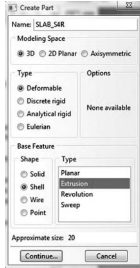
FIGURE 11.15 Creating the Slab_S4R Part.
