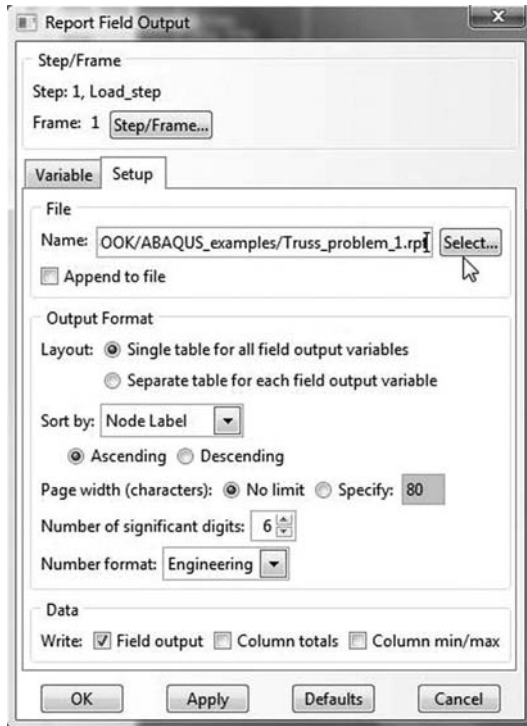
FIGURE 2.61 Choosing a directory and the file name to which to write the report.
