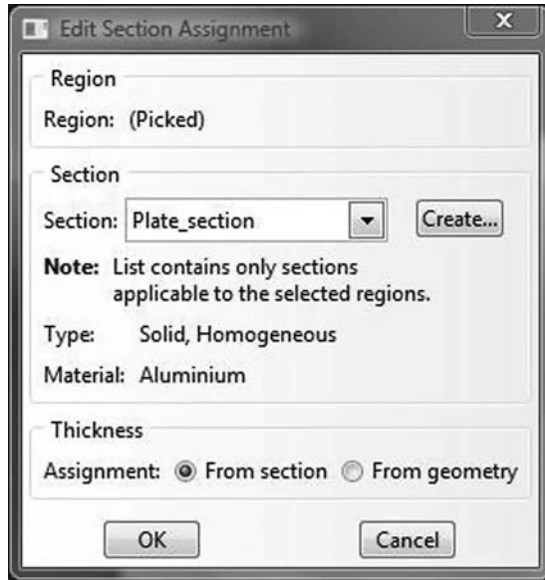
FIGURE 9.37 Editing section assignments.
