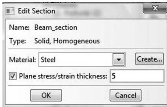
FIGURE 9.17 Creating a plane stress section.
