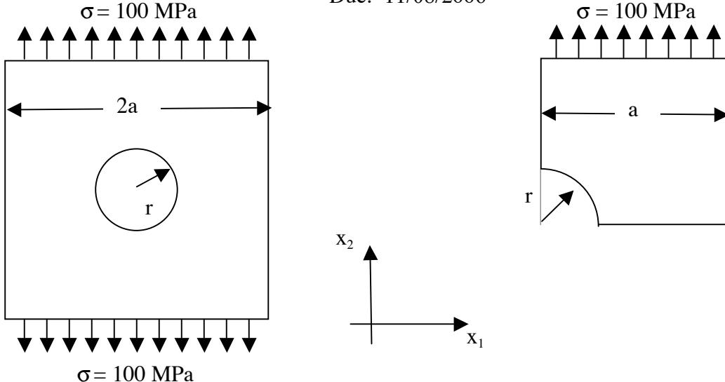
A square plate with sides length  $2a$  and a circular hole with radius  $r$  is shown above. The plate is under remote tensile loading,  $\sigma$ , as shown. A finite element model of the figure on the figure on the right, which takes advantage of the symmetry, is given in the input file *strnrhl-elps.inp* (see the end of this assignment for input file).
