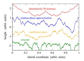
Fig. 2 Line scans of different surface realizations
