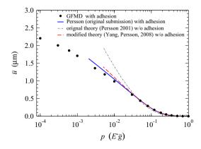
Fig. 1 Mean gap as a function of pressure as reported in Fig. 12 of the Contact-Mechanics Challenge [2] for the GFMD reference data and Persson's submission. Two new data sets are included, for which adhesion was not included
