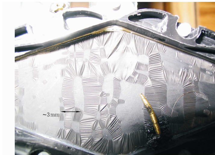
Fig. 14. An experimental observation of electromechanical instability (courtesy of Plante J. S. and Dubowsky S.). A layer of a dielectric elastomer, coated with conductive grease on top and bottom faces, is pre-stretched using a frame. An electric voltage is applied between the two electrodes. The layer deforms into a mixture of two regions, one being flat and the other wrinkled.
