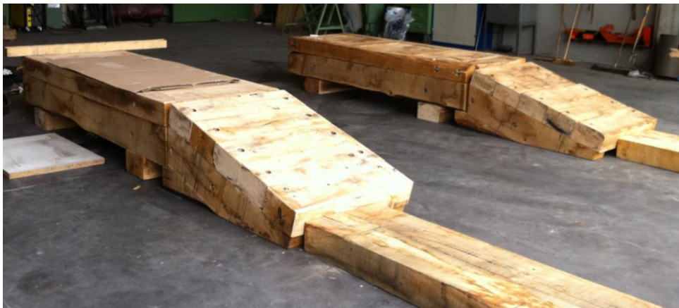
Figure 5 - Field Testing Setup to measure tread deformation
