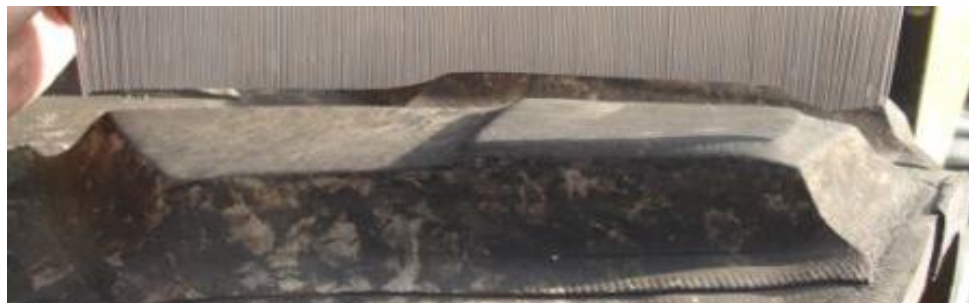
Figure 4 - Localized tread wear
