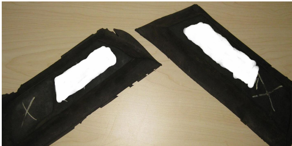
Figure 8 - Left side and Right side treads, with the severe worn areas marked in white, and the less worn areas marked with an "X"
