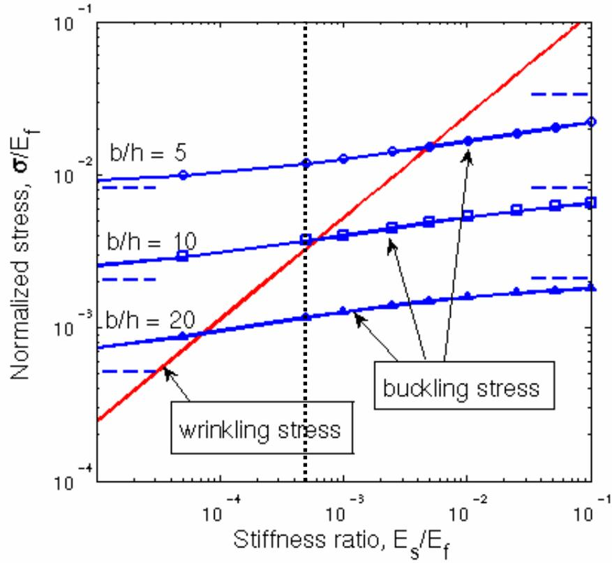
Fig. 2: (Color online) Comparison between the critical stresses for wrinkling and buckle-delamination. The open symbols are numerical results from Eq. (3) for various  $b/h$  ratios. The dashed lines indicate the limiting stresses for buckle-delamination. The vertical line represents the PS/PDMS system with  $\bar{E}_s / \bar{E}_f = 0.0005$ .
