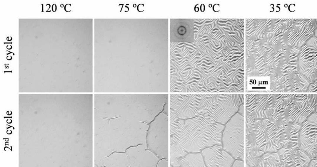
Fig. 4: Optical micrographs of a 120 nm PS thin film on a PDMS substrate cooled from 120 °C to room temperature, where wrinkling is the favored buckling mode during the 1<sup>st</sup> cooling cycle (top row) and buckle-delamination is favored in the 2<sup>nd</sup> cycle. The Fourier spectrum at 60 °C (inset) in the first cycle shows a well-defined wrinkle wavelength.
