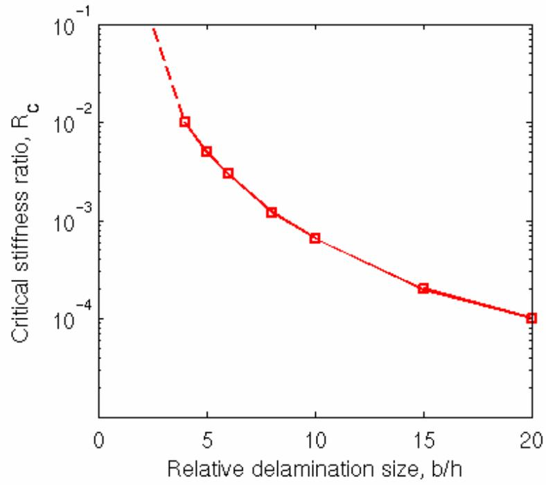
Fig. 3: The critical stiffness ratio as a function of the relative delamination size. Below the line, wrinkling is favored; above the line, buckle-delamination is favored. The dashed portion shows the qualitative trend beyond the limit of the plate theory used in deriving Eq. (3).
