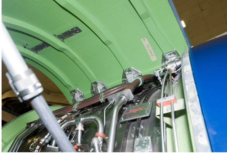
Figure 3. Metallic hinges attaching the composite fan cowl to the main structure
