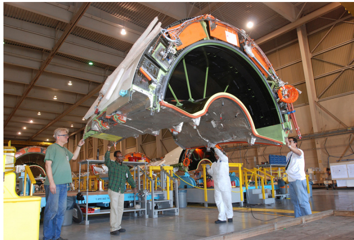
Figure 2. Goodrich thrust reverser for the Boeing 787 Dreamliner
