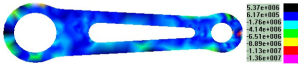
Fig. 12. Distribution of normal stress \sigma_x .
