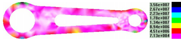
Fig. 13. Distribution of Von-Mises stress.
