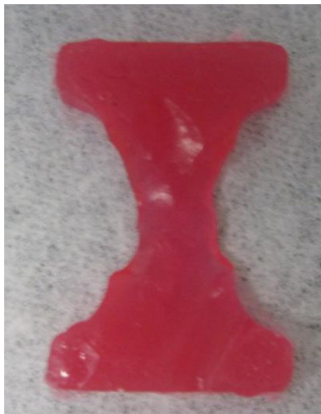
Fig. 2 – Picture of an Eco-flex 10 Platinum Cure Silicon Rubber sample with arbitrary shape.
