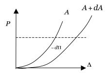
**Linear elasticity**. When the body is linearly elastic, the applied force P is linear in the displacement  $\Delta$ . Consequently, the elastic energy is
