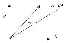
Compliance of a linearly elastic body containing a crack. For a linearly elastic body, the displacement is linear in the load. Write  $\Delta = CP$ ,
