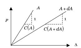
**Recover the Griffith result.** The energy release rate can be determined by solving a boundary-value problem in linear elasticity. Consider the Griffith crack (i.e., a crack of length 2a, in an infinite plate of unit thickness, subject to a remote stress  $\sigma$ ). The boundary-value problem was solved by Inglis (1913). The crack opens to the shape of an ellipse, and the opening displacement is
