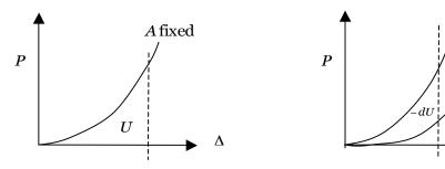
**Energy Release Rate**. Now consider two copies of the body: one copy has a crack of area A, and the other copy has a crack of area A+dA. The copy with the larger crack is more compliant—that is the load-displacement curve of the body with the larger crack is below the load-displacement curve of the body with the smaller crack. Consequently, at the same displacement, the body with a larger crack has lower elastic energy:
