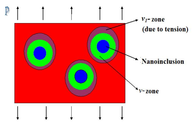
Under loading an additional zone with changed properties, which is called a prefracture zone, appears around the inclusion (*v* -zone ).
