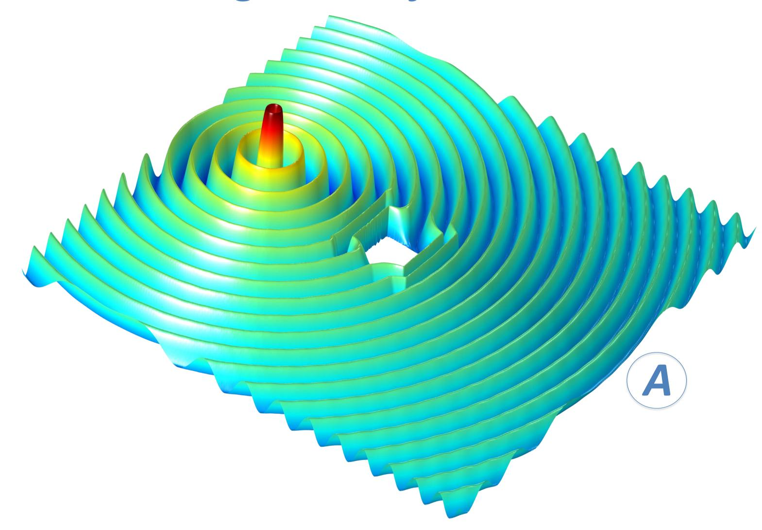
Using transformation elastodynamics, an exact cloak for bending waves in a Kirchhoff plate is created by a precise combination of an orthotropic elastic material and the application of pre-stress and body forces
