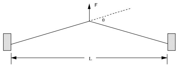
(b) The string typically vibrates with very small amplitude: there is negligible additional elongation of the string due to the vibration. Consequently, the tensile stress  $\sigma$  is constant during vibration. Furthermore, when the deflection *w* is small, the slope is given by  $\phi = \partial w / \partial x$ . Use a free body diagram of a spring segment dx to show the equation of motion:
