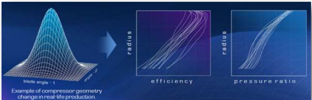
Fig. 1 Stochastic distribution of compressor efficiency indexes due to geometry variations
