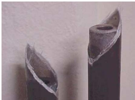
FIG. 7—Typical failure mode of the composite tube in a multi-axial fatigue experiment, showing failure is in the 45° plane to the specimen axis.
