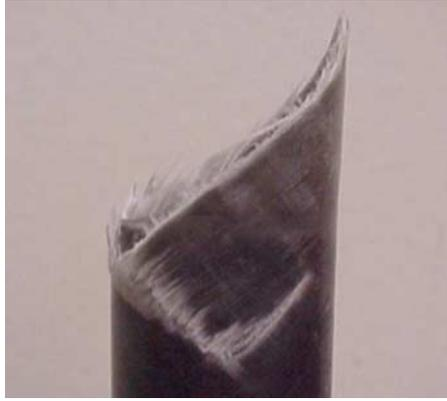
FIG. 5—Typical failure mode of a composite specimen from a monotonic multi-axial test.
