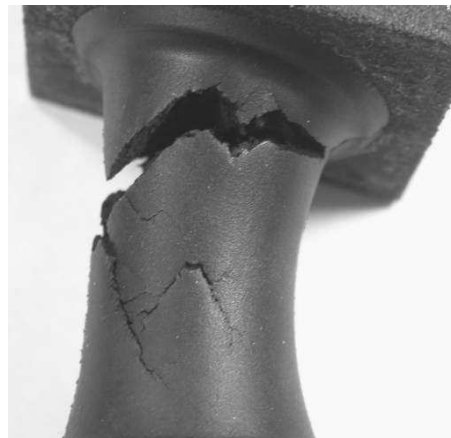
Fig. 6. Branching in the centre of the sample (non-relaxing uniaxial tension loading condition, maximum strain level \varepsilon_{max}^3 , R^3 = 0.29 ).
