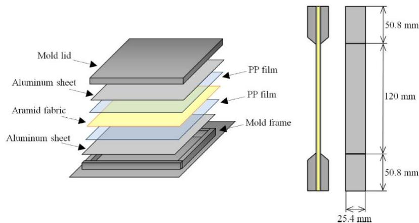
Figure 1: Construction of a typical fibre-metal laminate (left), and tensile specimen (right).
