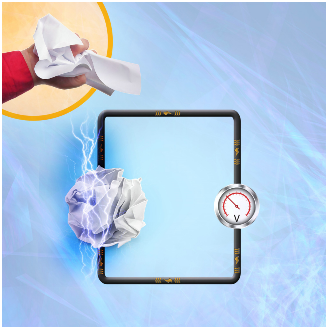
FIG. 1. Schematic of the electricity generated due to the crumpling of a thin dielectric sheet. Large strain gradients at the sharp tips in the crumpling sheet may polarize the material due to the phenomenon of flexoelectricity.
