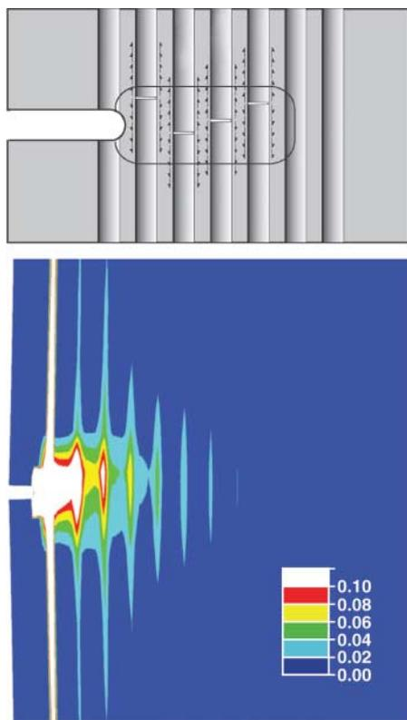
**Fig. 4.** Simulation of a metal matrix composite failing in bending: stochastic fiber breaks and interfacial sliding (**top**) and accumulated plastic strain (second strain invariant—scale given in key) in the matrix (**bottom**) (49).
