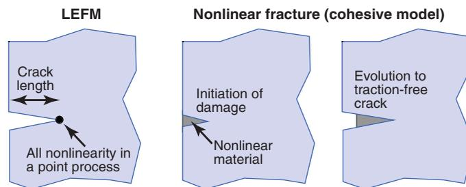
**Fig. 3.** According to linear elastic fracture mechanics (LEFM), the applied load required to evolve damage (grow the crack) tends to infinity as the crack length approaches zero. In a cohesive model, the applied load for damage initiation and evolution is limited to some finite multiple of the maximum value  $p_{\max}$  of a component of the assigned cohesive law  $\mathbf{p}(\mathbf{u})$ .
