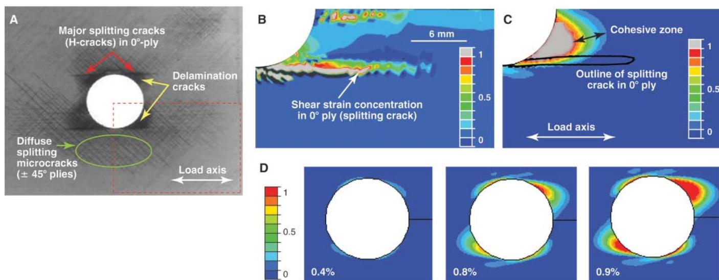
**Fig. 2.** (A) Images similar to Fig. 1 for a laminate that also contains angled ( $\pm 45^\circ$ ) fiber plies and a circular hole instead of a slit (23). The splitting cracks are now shorter, the delaminations are no longer wedge-shaped but lobe-shaped, and diffuse microcracking occurs predominantly in the  $\pm 45^\circ$  plies. (B) Computed continuum damage distribution in  $0^\circ$  ply (blue undamaged; gray is completely
