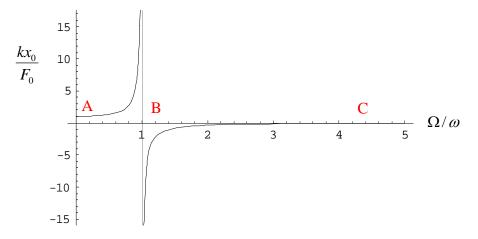
**Three behaviors of forced vibration.** Let us focus on the steady solution:
