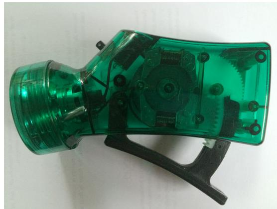
**Demonstration.** Bring a generator to class. The movement of my hand rotates a disk. The rotation induces an electric current in an electric circuit. The electric current lights up a bulb.
