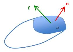
**Stress**. For a body in a homogeneous state, how many independent quantities do we need to calculate traction in a planar region of any direction? The answer is six. To see this answer requires a deeper generalization than the definition of traction.
