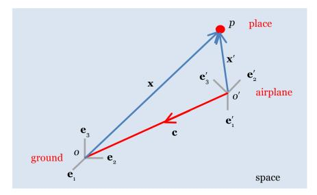
**Coordinates of a place.** The radial vector **x** is a linear combination of the base vectors,  $\mathbf{x} = x_i \mathbf{e}_i$ , where  $x_i$  are the coordinates of the place of the particle relative to the ground frame. Recall that  $\mathbf{e}_i = Q_{ai} \mathbf{e}'_a$ . Write  $\mathbf{x} = Q_{ai} x_i \mathbf{e}'_a$ . Now **x** is the radial vector of the place *p* from the ground origin, but  $Q_{ai} x_i$  are the components of the vector **x** relative to the airplane basis.
