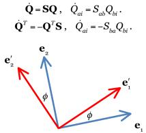
**Spin around an axis**. Consider a special case. At a given time, the two frames coincide, but the airplane rotates relative to the ground around  $\mathbf{e}_3$ . Let the angle of rotation be  $\phi(t)$ . The two sets of base vectors relate as
