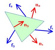
We have confirmed that the function  $\mathbf{f} = \mathbf{T}(\mathbf{a})$  is a linear map that maps one vector (the area vector) to another vector (the force). In linear algebra, such a linear map is called a tensor. In mechanics, we call this linear map the stress. Plasticity
