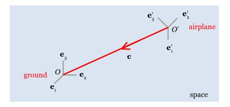
A base vector attached to the airplane,  $\mathbf{e}'_a$ , is a linear combination of the base vectors attached to the ground,  $\mathbf{e}'_a = Q_{ai}\mathbf{e}_i$ . Similarly, a base vector attached to the ground,  $\mathbf{e}_i$ , is a linear combination of the base vectors attached to the airplane,  $\mathbf{e}_i = Q_{ai}\mathbf{e}'_a$ . The two expressions together give that  $\mathbf{e}'_a = Q_{ai}Q_{bi}\mathbf{e}'_b$ . Any vector is a unique linear combination of the base vectors, so that
