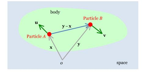
**Velocity gradient**. At a given time, particle *A* occupies a place of radial vector **x** and moves at velocity **u**, while particle *B* occupies a place of radial vector **y** and moves at velocity **v**. The two particles have the separation  $\mathbf{y} - \mathbf{x}$  and the relative velocity  $\mathbf{v} - \mathbf{u}$ .
