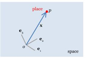
Let *p* be a place in the Euclidean space. Denote the separation from place *o* to place *p* by **x**, and call this separation the *radial vector*. The radial vector is a linear combination of the three base vectors,  $\mathbf{x} = x_i \mathbf{e}_i$ . The coefficients  $x_i$  are called the *coordinates* of the place *p* relative to the origin and the basis.
