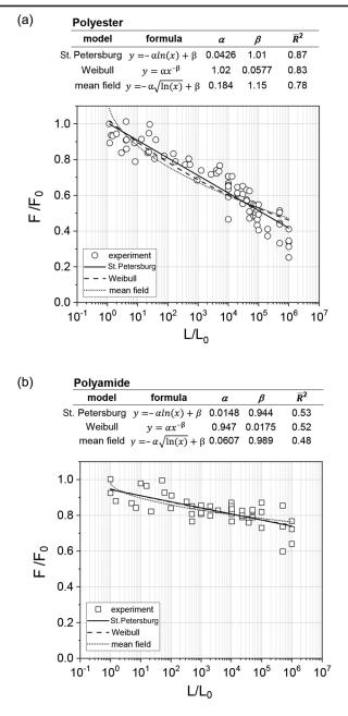
FIG. 2. Normalized fracture force for different length fibers. Normalized fracture force for the (a) polyester ( $L_0 = 1.2$  mm,  $F_0 = 17.84 N$ ) and (b) polyamide ( $L_0 = 1.0$  mm,  $F_0 = 42.60 N$ ) fibers as a function of fiber length from 1 mm to 1 km. The datasets were fit using the two parameter ( $\alpha, \beta$ ) St. Petersburg, Weibull, and mean-field models and are summarized in the tables above each graph.  $\bar{R}^2$  was used as a figure of merit.
