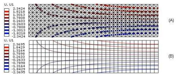
Fig. 4 Displacement contours in the x-direction of the cantilever: (A) the new element method; (B) the finite element method
