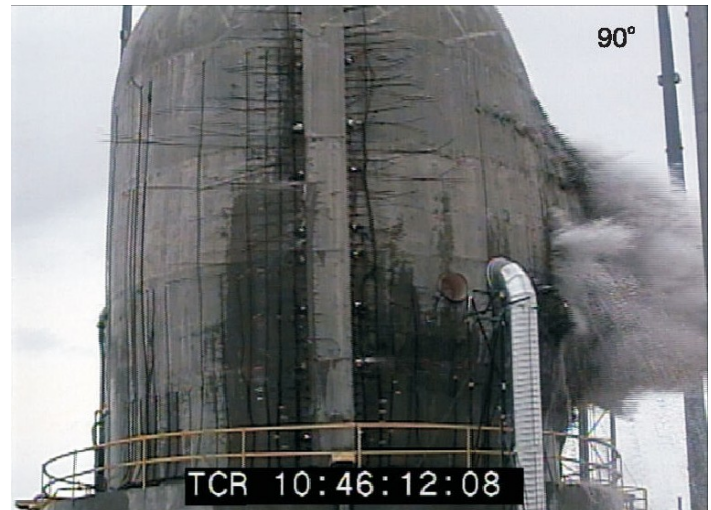
Figure 2: 1:4 scale PCCV prototype at the instant of structural failure (Ref. 1).
