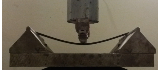
Figure 16: The experimental setup for the three-point bending test of an SMA beam.
