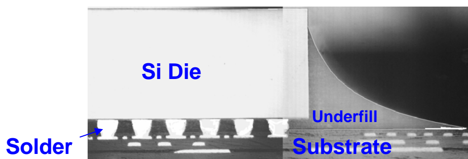
Fig. 2.2. Optical micrograph for the package cross-section used for moiré interferometry study.
