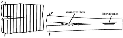
FIG. 2 Fiber pull-out.
