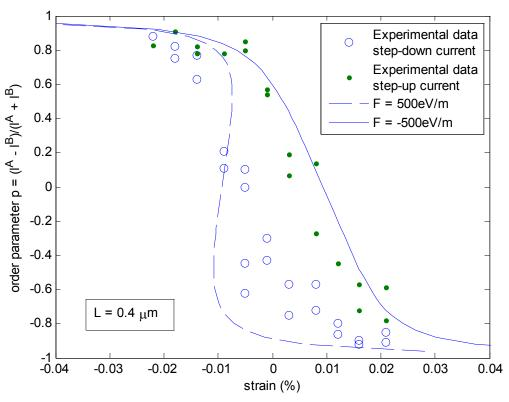
Fig. 4 In the stationary state, the relative terrace widths,  $p = (l^A - l^B)/(l^A + l^B)$ , is a function of the applied strain. The experimental data are taken from Tamura et al. (1997), carried out at 600°C and electric current density of  $10^6 \, \text{A/m}^2$ . The curves are the predictions of our model. (a) The average terrace width  $L = 0.12 \, \mu \text{m}$ .
