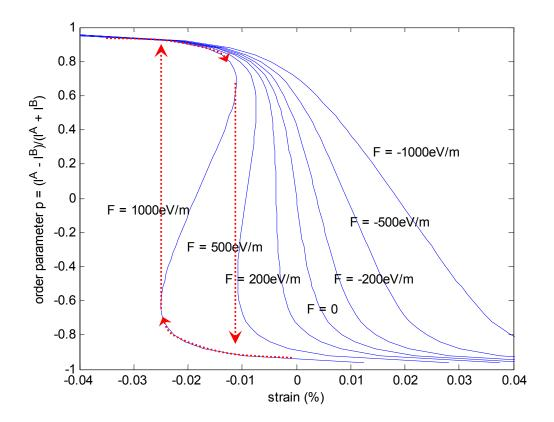
Fig. 5. The relative width of the terraces,  $p = (l^A - l^B)/(l^A + l^B)$ , as a function of the applied strain and the wind force. When the wind force blows step-down and is sufficiently high, e.g.,  $F = 1000 \, \text{eV/m}$ , the stationary state has an instability, in which a small change in the applied strain may lead to a large change in the relative width of the terraces. The dotted lines with arrows indicate a hysteresis loop.
