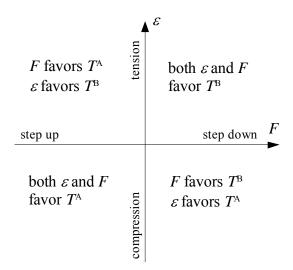
Fig. 3 Depending on the sign of the applied strain  $\varepsilon$ , and the direction of the wind force F, they can act either in concert or in competition to set a ratio of the widths of two variants of terraces.
