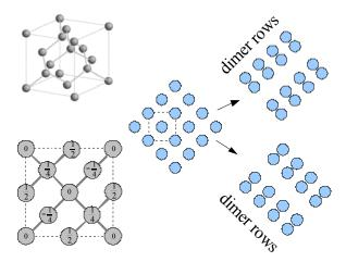
Fig. 1 Silicon has the crystalline structure of diamond. Upon reconstruction, atoms on the surface pair into dimers, which in turn form rows. Depending on the exact atomic plane, the dimer rows can be in either one of two directions.
