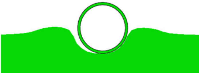
Figure 5: Soil berms and the partial embedment of the pipe after being cyclically displaced
