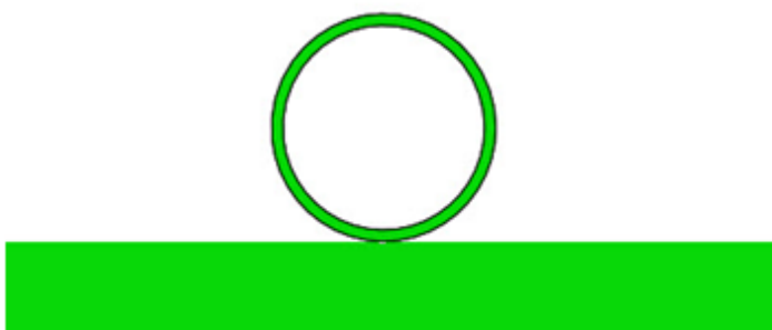
Figure 2: Initial configuration of the pipeline and seabed model for the CEL analysis
