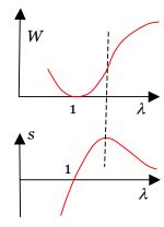
prescribed stress is below the peak, two states of equilibrium exist. Of the two states of equilibrium, the one with smaller stretch is stable, but the one with larger stretch is unstable. This statement can be verified by checking the sign of  $d^2W(\lambda)/d\lambda^2$ . Part of the function  $W(\lambda)$  is convex, and the other part is concave. The inflection point on the  $W(\lambda)$  curve corresponds to the peak on the  $s(\lambda)$  curve.
