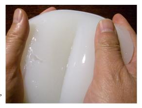
has been analyzed recently by E. Hohlfeld and L. Mahadevan (Phys. Rev. Letts. 106, 105702, 2011) In creasing, the amplitude of the field deviates greatly from the homogenous state, even though the spatial extent of an initial crease can be small. This mode of instability can also be analyzed by minimizing the free energy (Hong, Zhao, Suo, Applied Physics Letters 95, 111901, 2009, http://www.seas.harvard.edu/suo/papers/221.pdf).
