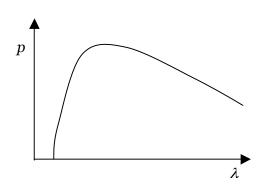
supply air at a constant pressure. When the balloon expands significantly, the pressure drops. Second, when the stretch is large, the rubber may stiffen significantly, at a rate much higher than that described the neo-Hookean model.
