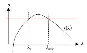
**Effect of strain rate on necking.** At an elevated temperature, glass flows and can be drawn into a thin fiber without forming necks. The rate-dependent deformation also has significant effect on the stability of metals even at the room temperature. Metals appear to be harder when they are loaded at a higher strain rate. A material model capturing this effect of strain rate is
