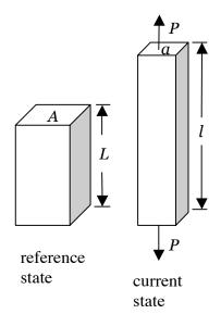
increment in the strain,  $\delta \varepsilon$ , as the increment in the length of the bar divided by the current length of the bar, namely,
