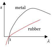
When a material undergoes large deformation, volumetric strain is often negligible compared to tensile strain. Consequently, such a material may be taken to be incompressible.
