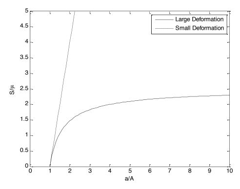
Sketch this result and compare it with the Lame solution, which assumes Hookean material and infinitesimal deformation. The cavity can expand indefinitely when the remote stress is still finite. The remote stress needed to cause the cavity to expand indefinitely  $(a/A \rightarrow \infty)$  is called the **cavitation limit**,
