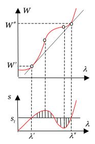
The bar is subject to an axial force of a fixed magnitude P. The bar and fixed force together are regarded as a composite thermodynamic system. In the current state, the Helmholtz free energy of the composite is
