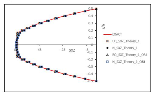
The transverse shear stress is computed based on Equivalent Single Layer Theory concept. Constitutive law is not used to compute it. The shear stress continuity condition is not imposed in the formulation a priori. No additional computation effort is required to estimate the stress distribution. The efficiency of the theory is excellent for thin and moderately thick beams and for thick beams, the values of the stress are very accurate (about 4%) at the interfaces.
