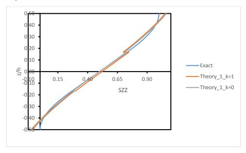
The transverse normal stress is computed based on Equivalent Single Layer Theory concept using constitutive law. The normal stress continuity condition is not imposed in the formulation a priori. The efficiency of the theory is excellent for thin and thick beams and the values of the stress are very accurate (about 6%).
