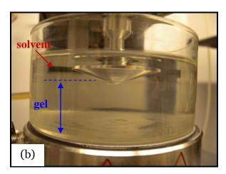
FIG. 3. Experimental setup. (a) A conical indenter made of aluminum. (b) The indenter is pressed into a disk of PDMS, which is submerged in a solvent.
