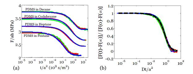
FIG. 6. A conical indenter was pressed to three depths into four disks of PDMS submerged in different solvents. (a) The force is normalized as F/ah, and the time is normalized as  $t/a^2$ . (b) The force is normalized as  $[F(t)-F(\infty)]/[F(o)-F(\infty)]$ , and the time is normalized as  $Dt/a^2$ . For the experimental data to fit the function  $g(\tau)$ , each solvent needs a distinct value of D, as listed in Table 2.
