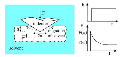
FIG. 1. A disk of a gel is submerged in a solvent throughout the experiment. Prior to indentation, the gel imbibes the solvent and swells to a state of equilibrium. An indenter is then rapidly pressed into the gel, and is subsequently held at a fixed depth h. The indenter causes the solvent to migrate in the gel, so that the force F on the indenter decreases as a function of time, until the gel reaches a new state of equilibrium.
