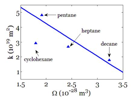
FIG. 9. Correlation between molar volume of solvent and diffusivity of the solvent in PDMS.
