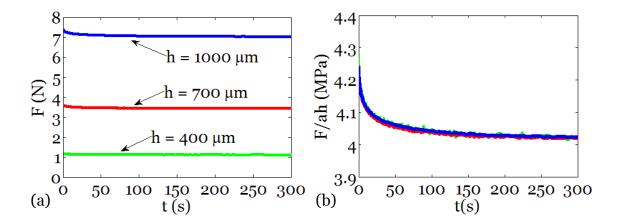
FIG. 2. A conical indenter was pressed into a dry PDMS sample to three depths. (a) Experimentally measured force as a function of time. (b) When the force is normalized as F/ah, but the time is not normalized, the force-relaxation curves for the three depths of indentation collapse to a single curve.
