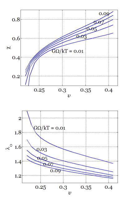
FIG. 7. Thermodynamic parameters are expressed in poroelastic parameters. (a) Flory-Huggins interaction parameter  $\chi$  vs. Possion's ratio v for various normalized shear modulus  $G\Omega/kT$ . (b) Swelling ratio  $\lambda_o$  vs. Possion's ratio v for various  $G\Omega/kT$ .
