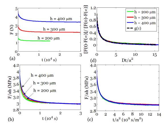
FIG. 5. A spherical indenter was pressed to three depths into a PDMS gel submerged in heptane. (a) Experimentally measured force as a function of time. (b) The force is normalized as F/ah, but the time is not normalized. (c) The force is normalized as F/ah, and the time is normalized as  $t/a^2$ . (d) The force is normalized as  $[F(t)-F(\infty)]/[F(0)-F(\infty)]$ , and the time is normalized as  $Dt/a^2$ .
