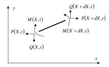
*Momentum balance*. If we make an imaginary cut at a cross section of the elastica, we expose an internal moment M(X,t), and a pair of internal forces P(X,t) and Q(X,t) along the directions of the two axes. You may project the forces along, and normal to, the tangent direction, and call them axial and shearing forces, but we will not do so here.
