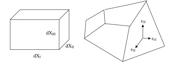
Hyperelastic material. Let  $WdV(\mathbf{X})$  be the elastic energy stored in an element of volume in the current state. When the deformation gradient changes by  $\delta F_{iK}$ , the stress does work  $s_{iK}\delta F_{iK}$ . Assume that all this work is stored as the elastic energy in the particle, so that
