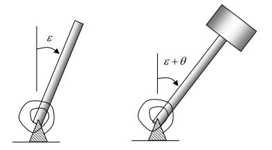
One way to introduce an imperfection is to assume that in its unloaded state, the spring is installed such that the rod has some initial deviation  $\varepsilon$  from the vertical position. Thus, the energy function becomes
