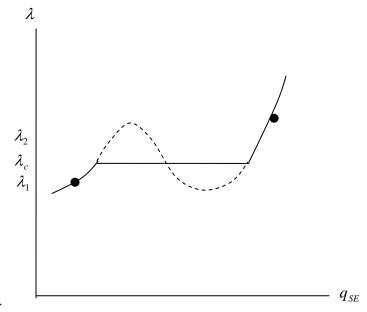
family of systems with the following characteristics. When  $\lambda < \lambda_c$ , the system has a minimum. As  $\lambda$  increases gradually, the depth of the minimum becomes smaller and smaller. Then a critical value  $\lambda_c$  is reached, such that the local minimum disappears. In this situation, there will be no energy barrier for the system to switch configuration.
