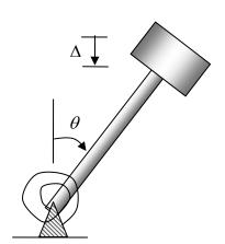
In general, for a system of one degree of freedom, we specify the configuration of the system with a generalized coordinate q, which is a parameter uncontrolled and free to vary. The free energy of the system is a function of the generalized coordinate, G(q). A stable equilibrium configuration corresponds to a generalized coordinate that minimizes the free energy.
