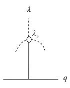
Subcase d < 0. For a member system with  $\lambda < \lambda_c$ , the configuration q = 0 is a local minimum, and the nontrivial equilibrium configurations correspond to two maxima. For a member system with  $\lambda > \lambda_c$ , the configuration q = 0 becomes a maximum. This kind of instability is called *unstable bifurcation*.
