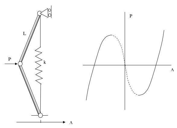
Critical point of configurational transition of the second type. Bifurcation analysis. Let us focus on configurational transitions of the second type, and summarize the procedure to determine the equilibrium configuration and critical point. The analysis is local, so that each minimum is understood to be a local equilibrium and corresponds to a metastable configuration. We will not always explicitly mention the words local and metastable.
