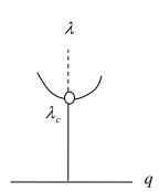
Subcase d>0. For a member system with  $\lambda<\lambda_c$ , the configuration q=0 is a local minimum. For a member system with  $\lambda>\lambda_c$ , the configuration q=0 is a local maximum, but two new local minima emerged. This kind of instability is called the *stable bifurcation*. Example: ferroelectric crystal.
