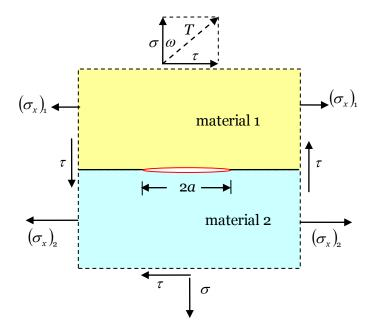
It may be tempting to choose the length of the crack, a, as the length l to define the mode angle. This choice goes against the spirit of fracture mechanics. We would like to use the mode angle to characterize the field near the tip of the crack. The same mode angle should mean the same local field. However, the length of the crack is a parameter that characterizes the geometry of the specimen.
