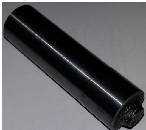
Fig. 3 Geometry of used tool during the process, (a) drawing of the tool, (b) shape of the real tool
