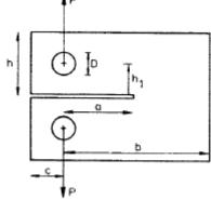
The bending and compact tension specimens can be used to determine the critical J for initiation of crack growth as well as the resistance curve J vs  $\Delta a$  for small amount of crack growth (Shih et al., 1978).
