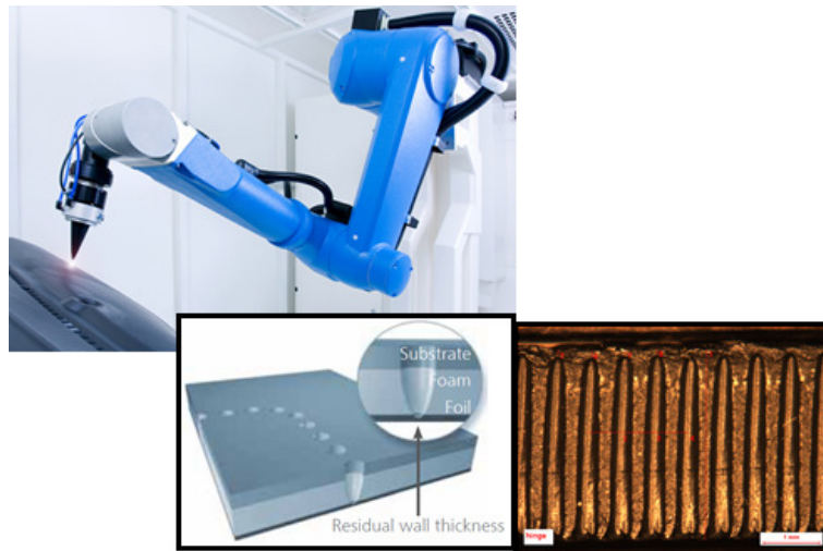
Figure 4. Micro holes created by a laser machine
