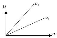
Let  $\lambda$  be a loading parameter, which can be an applied force, or a prescribed displacement. The energy release rate depends on both the loading parameter and the length of the crack, namely,
