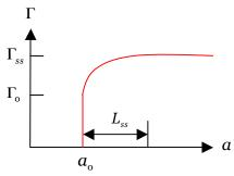
Under the small-scale yielding condition, the R-curve is a material property. The R-curve is independent of the initial length of the crack,  $a_{\rm o}$ . Nor does the R-curve depend on the geometry of the specimen. Parameters of importance include
