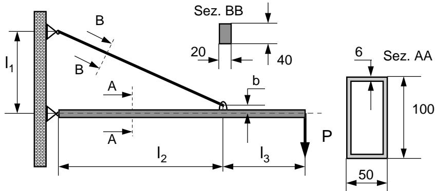
Dati:  $l_1 = 1 \text{ m}$ ;  $l_2 = 1.5 \text{ m}$ ;  $l_3 = 0.9 \text{ m}$      $b = 100 \text{ mm}$ ;  $P = 5 \text{ kN}$
