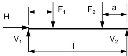
$$\begin{aligned} \rightarrow H = 0 \quad & V_2 = \frac{F_2(l-a) + F_1a}{l} = 15 \text{ kN} \\ 1 \supset V_2 l - F_2(l-a) - F_1a = 0 \quad & \Rightarrow \\ 2 \supset V_1 l - F_1(l-a) - F_2a = 0 \quad & V_1 = \frac{F_1(l-a) + F_2a}{l} = 15 \text{ kN} \end{aligned}$$
