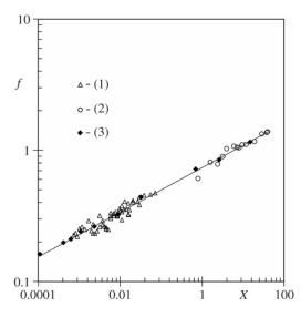
**Fig. 3.** Data collapse in coordinates  $f = M/\rho R^{2.48}$  (in arbitrary units) versus the geometric constraint  $X = Lh^{0.9}/W^{1.9}$  for randomly folded aluminum foils of different geometry: triangles —the square sheets (the data from Ref. [83], the same that used in Fig. 1), circles—the strips of width W = 2 mm from aluminum of thickness 0.02 mm (see Fig. 2), and rhombs—the strips of length L = 500 mm. The slope of fitting line is 0.17.
