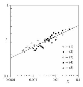
**Fig. 1.** Data collapse in coordinates  $f = M/\rho R^{2.48}$  (mm<sup>0.52</sup>) versus X = h/L (arbitrary units) for randomly folded foils (W = L) of thickness h = 0.02 (1), 0.06 (2), 0.12 (3), 0.24 (4), and 0.32 mm (5) studied in the work [83]. The slope of straight line is 0.15.
