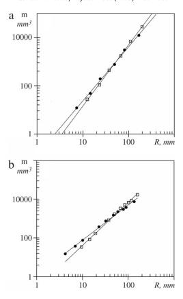
**Fig. 4.** Log-log plots of  $m = M/\rho = LWh \, (mm^3)$  versus  $R \, (mm)$  for sets of randomly folded papers: (a) sets of square sheets of thickness 0.03 (full circles) and 0.069 mm (squares); the slopes of fitting lines are  $D_2(3) = 2.25$  and  $D_2(3) = 2.54$ , respectively; (b) set of strips of length L = 500 mm from papers of thickness 0.03 mm (full circles) and 0.068 mm (squares); the slopes of fitting lines are 1.8 and 2.2, respectively.
