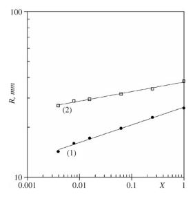
**Fig. 5.** The ball diameter R (mm) versus the geometric constrain X = W/L for the sets of randomly folded paper sheets of the mass  $M/\rho = 6400 \text{ mm}^2$  with the thickness h = 0.03 mm (1) and 0.068 mm (2); the slopes of straight lines are 0.12 (1) and 0.06 (2), respectively.
