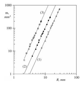
**Fig. 2.** Log-log plots of  $m = M/\rho = LWh \, (mm^3)$  versus  $R \, (mm)$  for sets of randomly folded strips of width  $W = 2 \, mm$  from papers of thickness 0.068 (1) and 0.03 mm (2) and aluminum of thickness 0.02 mm (3). The slopes of all fitting lines are equal to  $D_1(3) = 3 \pm 0.1$ .
