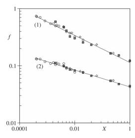
**Fig. 6.** Data collapse in coordinates  $f = M/\rho R^{D_2}$  (in arbitrary units) versus X = W/L for randomly folded sheets of paper of different geometries with the thickness h = 0.03 mm (1) and 0.069 mm (2): circles—the strips of width 2 mm (see Fig. 2), full squares—the strips of length 500 mm (see Fig. 4(b)), and rhombs—the strips with  $L \times W = \text{const}$  (see Fig. 5). The slopes of straight lines are  $D_2/D_1 - 1 = -0.24$  (1) and -0.15 (2).
