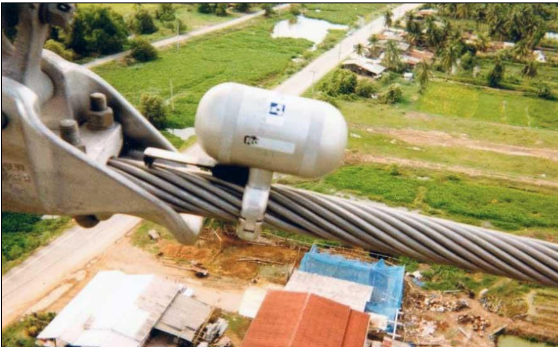
Fig. E-6. PAVICA Aeolian Vibrations sensor-analyser-recorder
