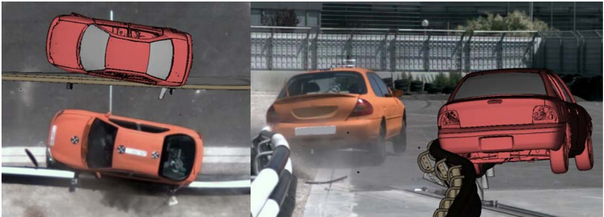
Figure 9. Maximum deflection during the test and simulation
