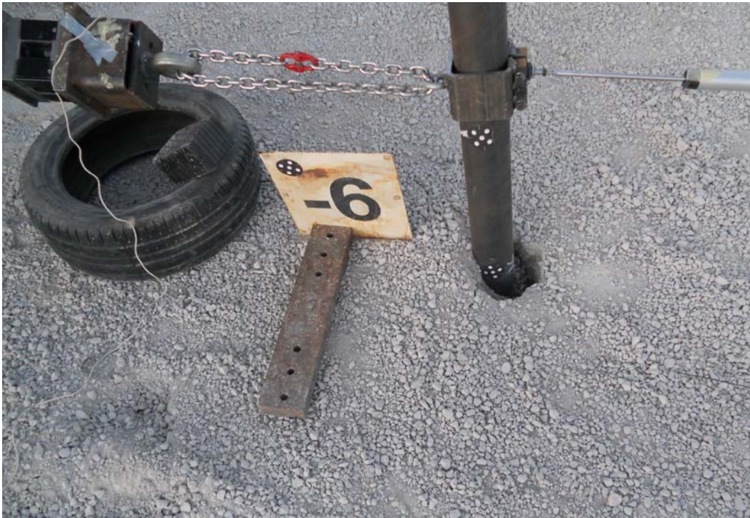
Figure 1. Configuration of a pole pull-out test
