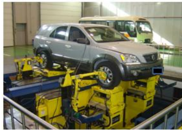
Figure 8. SPMD (suspension parameter measuring device)
