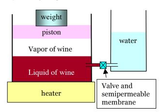
The function S(U,V,N) of a system. When we thermally insulate the wine, fix the position of the piston, and close the valve, the three variables of the wine, (U,V,N), are fixed at a particular set of values. Consequently, once (U,V,N) are fixed, the wine is an isolated system, flipping among a set of microstates. Let  $\Omega$  be the number of the microstates of the isolated system.
