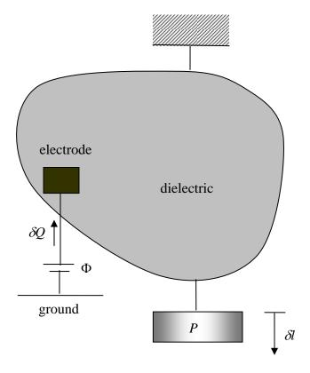
Figure 2 A dielectric is loaded by two mechanisms: a weight and a battery. When the weight drops by a displacement  $\delta l$ , the weight does work  $P\delta l$ . The dielectric is perfectly insulating, but battery can pump electric charges from the ground to the electrode. When the electrode gains charge  $\delta Q$ , the battery does work  $\Phi \delta Q$ .
