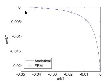
Fig. 4. A blanket layer of a gel is bonded to a rigid substrate and is in contact with a solvent. The gel swells in the normal direction (a), and develops an equal-biaxial compressive stress (b). The initial swelling is set to be  $\lambda_0 = 1.5$ .
