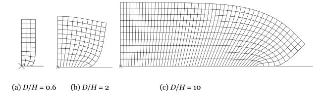
Fig. 7. The equilibrium configurations of the cylinders of several aspect ratios. In case (c) significant contact is observed between the side wall of the gel and the substrate.
