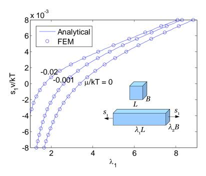
Fig. 3. A rod of a gel is subject to a uniaxial stress, and is in contact with a solvent of a given chemical potential. The applied stress is plotted as a function of the stretch, while the solvent is held at several levels of chemical potential.
