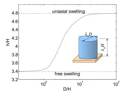
Fig. 6. A cylinder of a gel is bonded to a rigid substrate and is in contact with a solvent. The equilibrium height of the cylinder is plotted as a function of the aspect ratio of the dry polymer, D/H.
