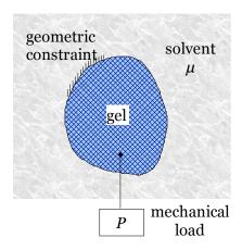
Fig. 1. A gel is in contact with a solvent of a fixed chemical potential, and subject to a mechanical load and geometric constraint.
