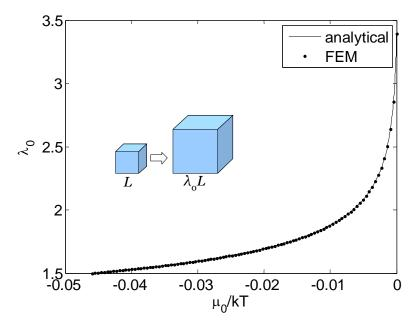
Fig. 2. The free-swelling stretch of a gel is plotted as a function of the chemical potential of the solvent molecules.
